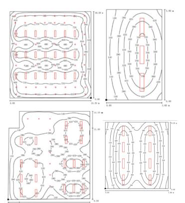
Figure 6. Distribution of artificial lighting illuminance (lux) for the following rooms: conference room at the fourth floor (top-left), reception at the second floor (top-right), open-plan office at the second floor (bottomleft), a private office (bottom-right).
