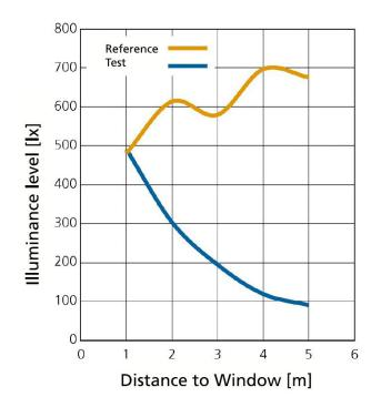
Figure 5. Horizontal illuminance on the working plane provided by electric lighting only. The illumination of the test room with light-emitting structures is provided by the structure only, which is located on the upper part of the window.
