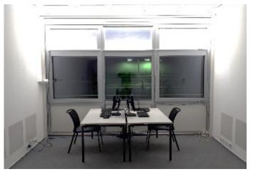
Figure 1. The lab room seen from the inside. The light-emitting structures are placed on the top part of the windows and provide illumination to the room interior.
